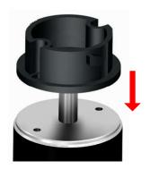
Set the base plate onto the motor
