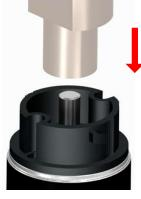
Align the base plate to the motor shaft by using the centering gauge
